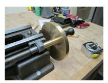
Now were off to making things, like a new handle for the lead screw. 4" diameter solid brass sure makes it easier to turn by hand. Along with purchasing a new tool post, some cutting tools, new brass gibbs for the tool post slide and compound swivel base.
